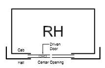
**Note:** For Center Opening use the direction of the driven door when closing
